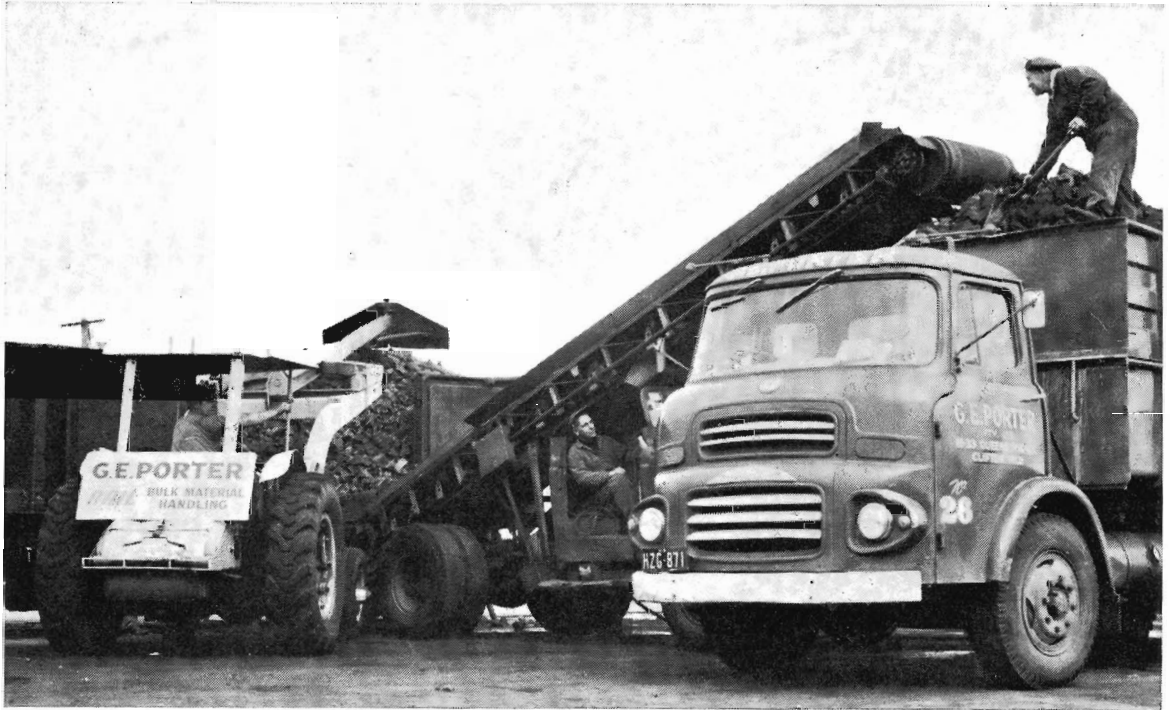
Rapid unloading of metallurgical coke at Dynon, by contractor's special equipment
