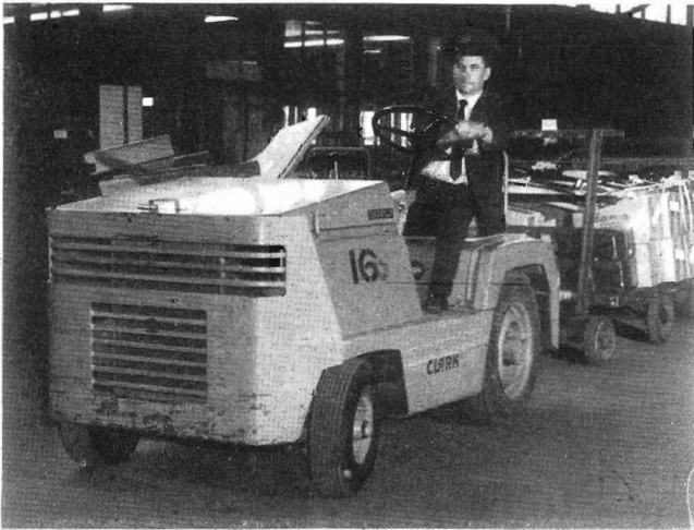
New LUGGAGE TRACTOR: The latest type of luggage tractor is this Clarkor that is being driven by Station Assistant D. Moody at Spencer Street. Its engine develops 68 b.h.p. at 2,650 r.p.m. and the drive, through hydraulic coupling, gives a smooth start.
