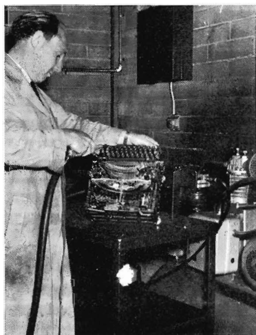
Typewriter Mechanic K. Brown uses compressed air to blow dust from machine before it is given a cleaning bath. (Rubber dust from type erasers mixes with the lubricating oil and makes the mechanism stick.)
