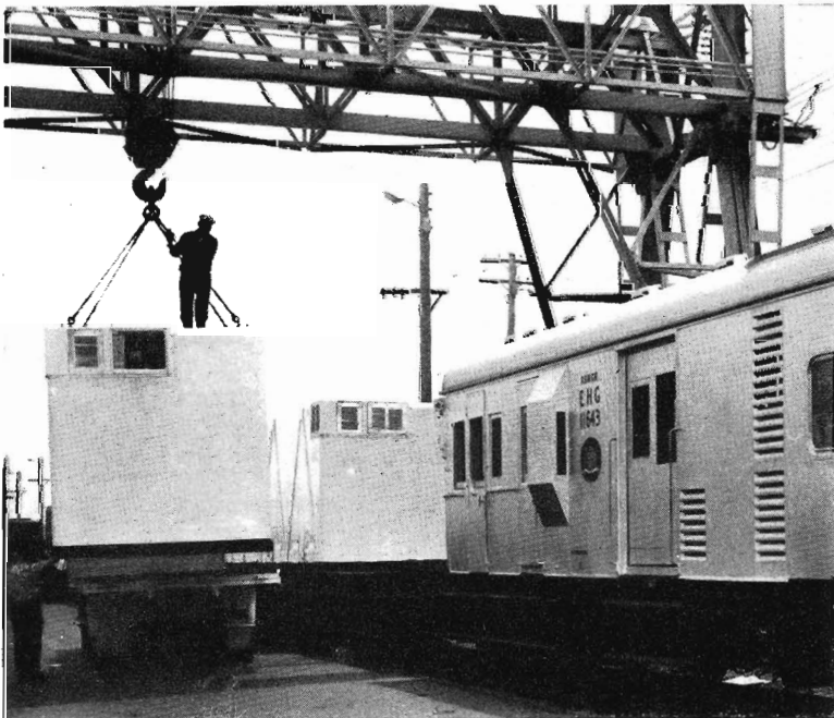
At Dynon, a container of frozen vegetables from Tasmania is being loaded from road vehicle on to flat-top rail wagon. The power van at right is supplying power for refrigerators in the containers.
