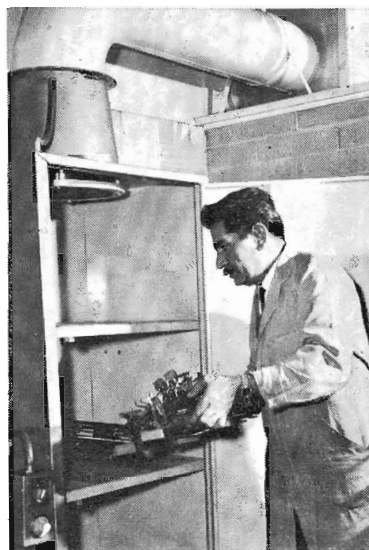
After the cleaning bath, typewriters are put into a drying cabinet where solvent from the bath is removed. Typewriter Mechanic E. Callas is shown placing a machine in the cabinet.
