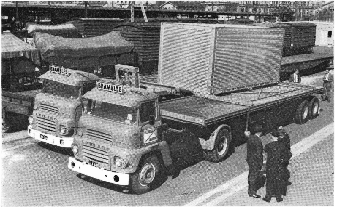
CONTAINERS SIDE-LOADED : A demonstration of side-loading of containers was recently given at Melbourne Goods. Picture shows the road transfer unit (left) unloading the container from the road transport. The transfer unit then loaded the container on to the rail wagon (not visible) at left of unit.
