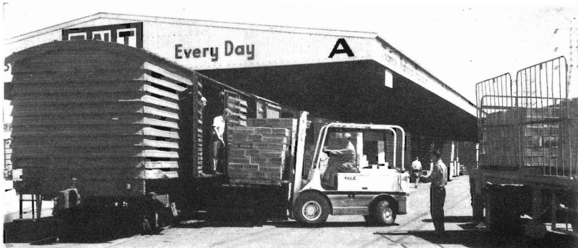
A fork lift truck transfers goods from Flexi-Flat to rail van in a section of the Forwarding Agents' area at North Dynon.
