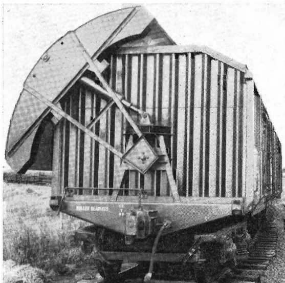
TAILORED TRANSPORT: Shown near the Sunshine factory of John Lysaght (Aust.) Ltd., this prototype N.S.W. Railways wagon has been specially designed to meet the needs of consignors of sheet steel in coils. As well as providing full protection for the goods in transit, the roof can be swung clear to enable loading of the steel by overhead crane. A manually operated hand wheel and reduction gearing enable the roof to be swung to either side of the wagon.
