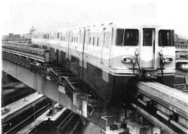
Six carriage Tokyo to Haneda monorail train passes through track switches as it enters Hamamatsu-cho station, Tokyo. At lower left are the J.N.R. suburban lines passing below the monorail track. (Photos: A. J. Nicholson)
