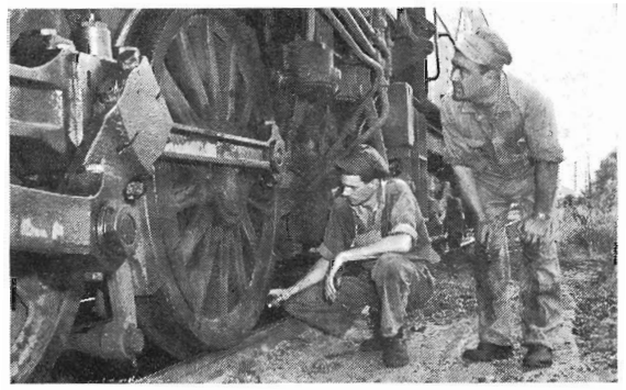
Fireman John Fowler (left) checks ash pan slides while Driver Don Harris looks over motion gear of J 522. Don has been at Horsham for nine years; John is a recent arrival there. The locomotive hauled the 7 a.m. goods ex Goroke.
