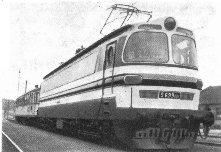
Polyester glass fibre is used in both cab and body of this new Czechoslovakian electric locomotive.
