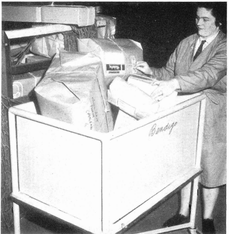
At the Outwards Parcels Office, Station Assistant Margaret Vergos loads one of the new mobile sorting bins that have recently been introduced. These bins eliminate unnecessary walking and carrying of parcels by the staff.
