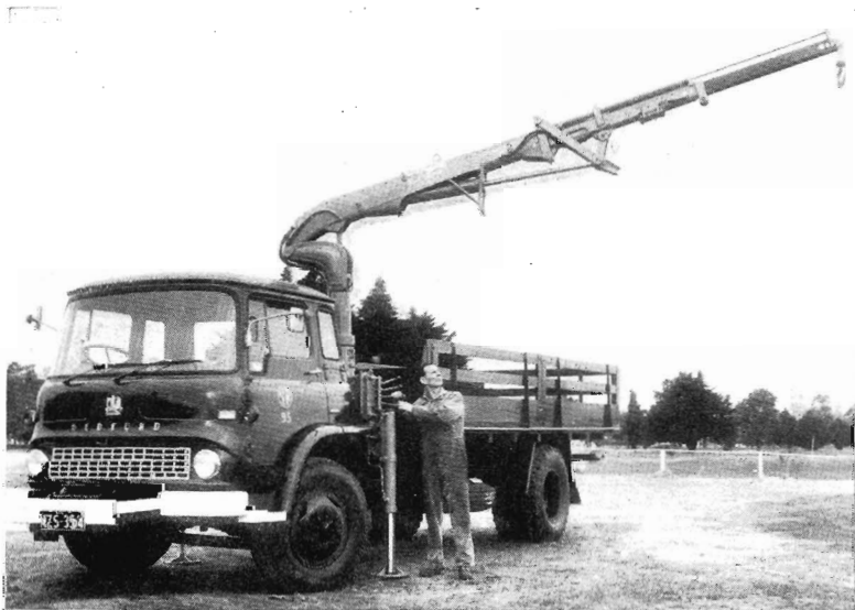
Leading Hand Mechanic Geoff Nixon tests the operating controls of a new Signal and Telegraph Division mobile crane. It has a maximum lift of 2½ tons, uses hydraulic power supplied by truck engine, and boom can be extended to 13 ft.
